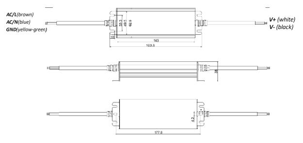
150W Constant Voltage LED Switching Power Supply
